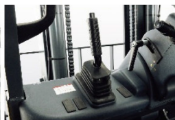
Ratchet type parking brake
