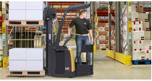
The NPV20PD double pallet handler with foldable platform saves time by carrying two pallets simultaneously (one above the other). It is perfect for double stacking on the loading ramp and for transporting incoming or outgoing loads over short, medium or long distances.
